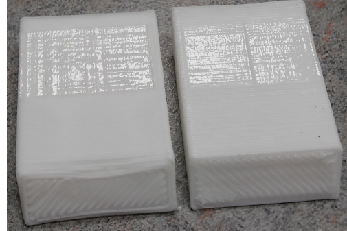
Figure 3: Blocks partly treated with the laser polishing process
